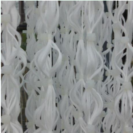
The surface of the carrier is designed to mimic plant roots
