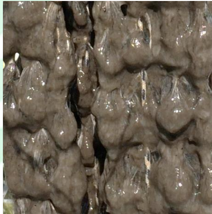
The carrier is able to support large quantities of biomass
